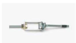
Option: Depending on system length 4 or 6 special ceiling mounting accessories (type DH/DHD) are screwed into blind rivet nuts on the top of the air curtain system and anchored into the ceiling above the door with heavy duty dowels. Adjusting of the turnbuckles allows horizontal alignment at the correct height.
